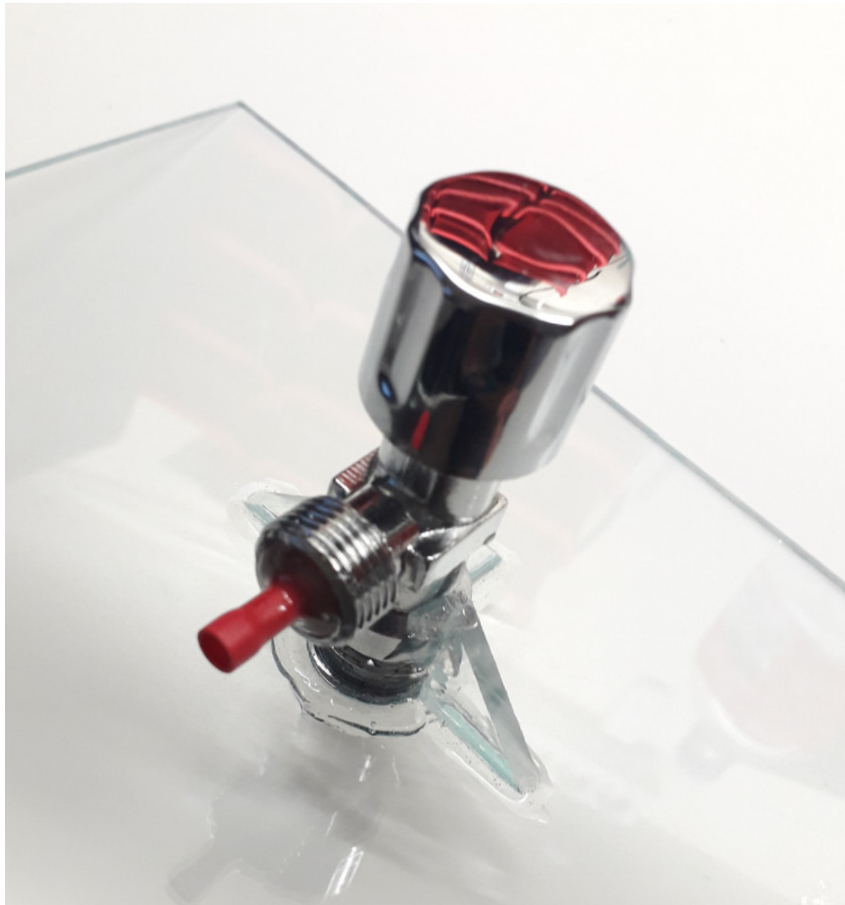
Out gas and pressure regulator
